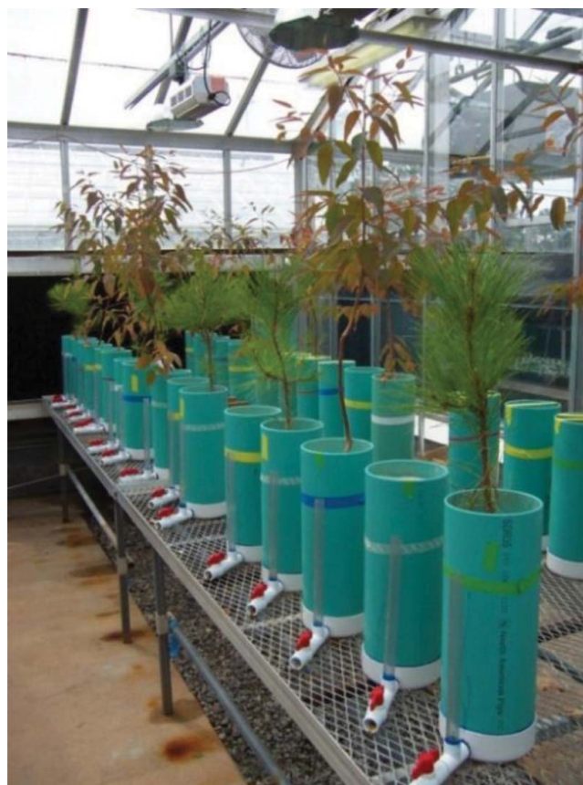
Figure 2. Greenhouse experimental setup containing eucalyptus (blue bands), pine (green bands), and no-plant controls (white striped bands) in the greenhouse.
